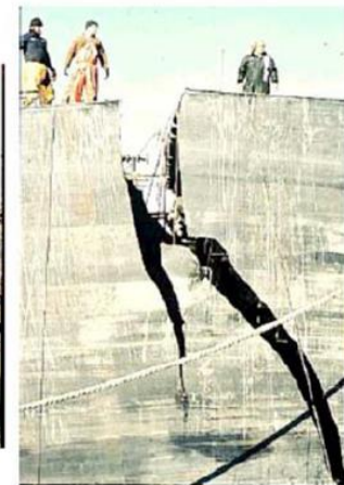
Brittle failure of Liberty ship during WW II
