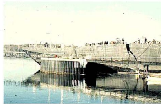
Brittle failure of Liberty ship during WW II
